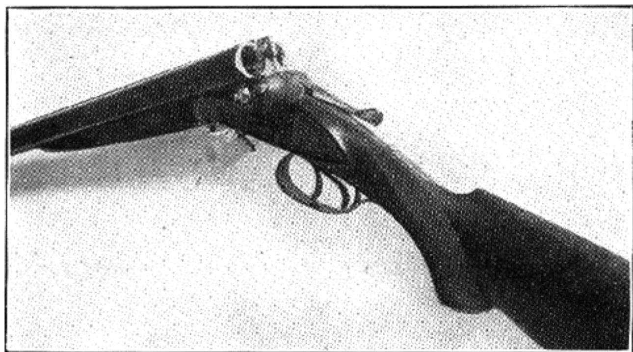
The Diamond Daly; beautiful German style of engraving considering strength alone, for a gun with long frame *must* outlast the one with short frame, other things being equal. This is for the reason that there will be less leverage against the locking bolts. It is true, however, that this rule works both ways, and if a short framed gun gives more leverage against its fastenings, it also exerts greater lever power in cocking both the main lock and the ejec-
